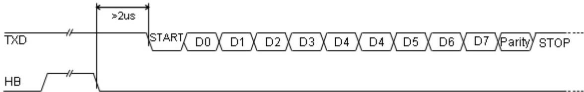
TTL Asynchronous serial communications from VFD module to host system
