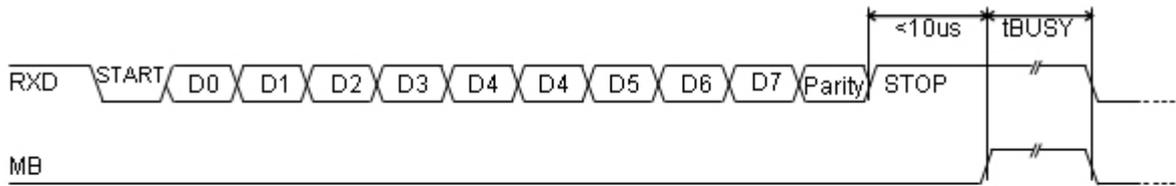
TTL Asynchronous serial communications from host system to VFD module
